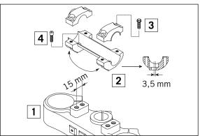
For this purpose, remove screws [3] of the handlebar clamps and screws [4] of the handlebar support. Position the handlebar support, and tighten screws [4] to 40 Nm (30 ft.lbs). Mount the handlebar and handlebar clamps, and tighten screws [3] to 20 Nm (15 ft.lbs). The gap between the handlebar support and the handlebar clamps should be the same size in the front and in the rear.
